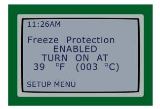
Freeze Protection can be either enabled or disabled when the user turns the User Interface selector knob to Setup. If it is enabled, the user will be able to set the temperature at which the pump will turn on. The control is designed to run the pump for 8 hours at 2600 RPM if the temperature drops below the setpoint.
