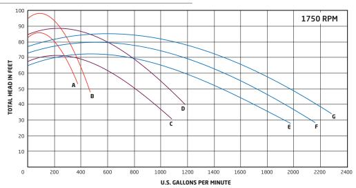
**A. Normblock Multi 65/250** (Ø 225mm) - 7.5 HP S.F. 1.25 **B. Normblock Multi 65/250** (Ø 240mm) - 10.0 HP S.F. 1.25 **C. Normblock Multi 100/250** (Ø 220mm) - 15.0 HP S.F. 1.25
