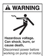
Pool pump must be installed by a licensed or certified electrician or a qualified pool serviceman in accordance with the National Electrical Code and all applicable local codes and ordinances. Improper installation will create an electric hazard which could result in death or serious injury to pool users, installers, or others due to electrical shock, and may also cause damage to property.
