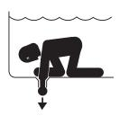
Pool and spa pumps produce high levels of suction, which can pose extreme danger if a person comes in close proximity to an open pool or spa drain or if a drain cover is loose, cracked, broken or missing. Pool and spa pumps move large volumes of water, which can pose extreme danger if a person's hair comes in close proximity to a drain that is not the proper size for the pump or pumps.
