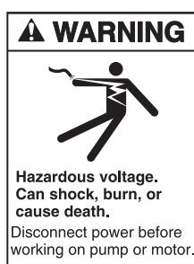
Pool pump must be installed by a licensed or certified electrician or a qualified pool serviceman in accordance with the National Electrical Code and all applicable local codes and ordinances. Improper installation will create an electric hazard which could result in death or serious injury to pool users, installers, or others due to electrical shock, and may also cause damage to property.
